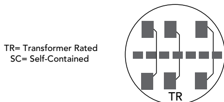
2 or 3 ELEMENT 3Ø3W, Y or Δ FORM 8S & 9S with bypass
